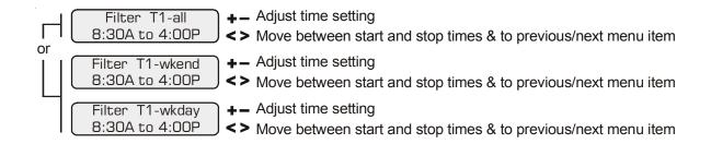
For one speed pumps, this is the first filter timeclock and will determine the normal hours of filtration for the pool. For pool/spa combination systems with spillover enabled, the valves will automatically switch to spillover mode at the start of the filtration period. For all other systems, the valves will switch to the pool-only position.
