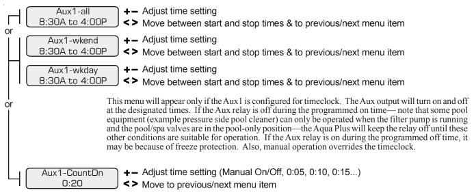
This menu will appear only if the Aux1 is configured for countdown timer. This setting is the time after you manually turn on the Aux relay until the Aqua Plus automatically turns off the relay. You can also manually turn off the relay at an earlier time by pressing the AUX1 button.
